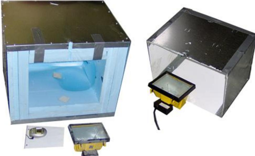
A fourth metal box was constructed with dimensions of 24"x24"x20" and lined with 4" of Styrofoam insulation to give it a R20 building code rating. It was significantly larger than the other metal boxes but has the same volume inside for air. A thermocouple was placed inside the box to measure the inside temperature of the box the same as the other three boxes.
