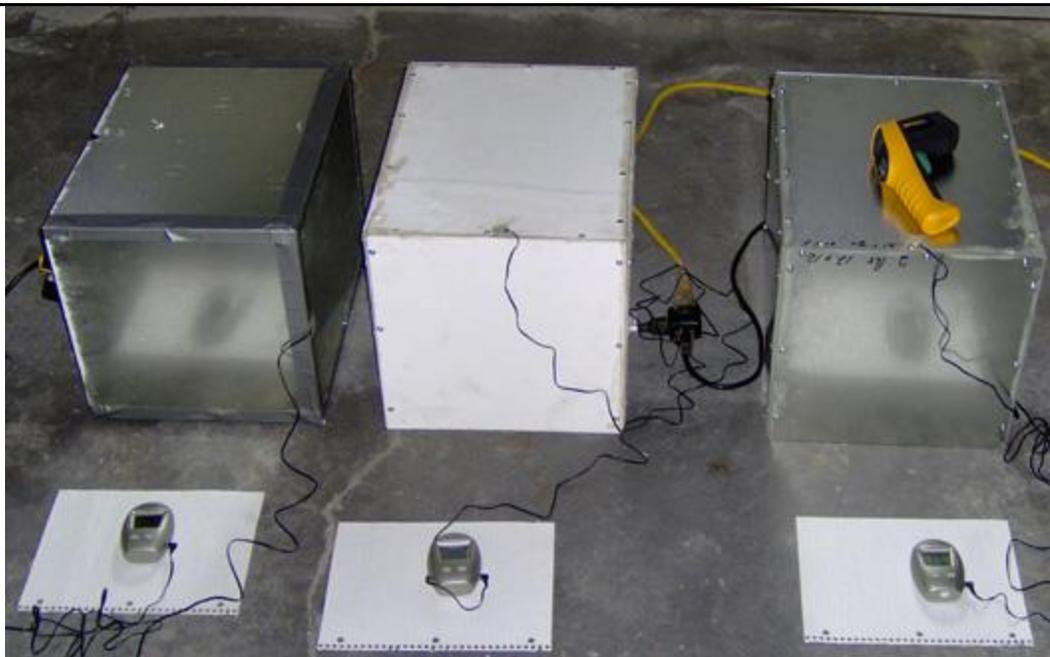
Three Metal boxes were constructed. Each metal box had the same dimensions of 12"x16"x16" so that the volume of each box was the same.
